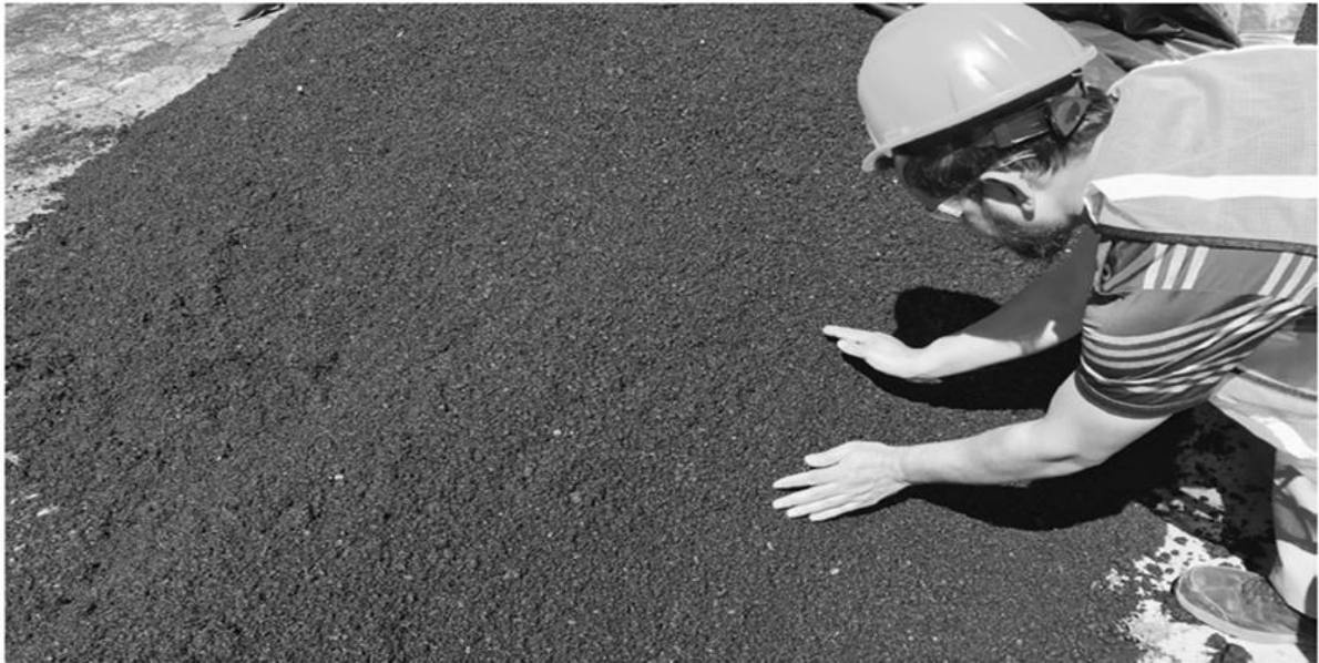
Figure 47 Cold Mix Asphalt
